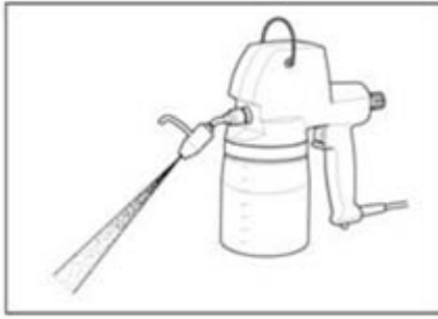
Nozzle handle upwards. Flushing with sharp jet.
